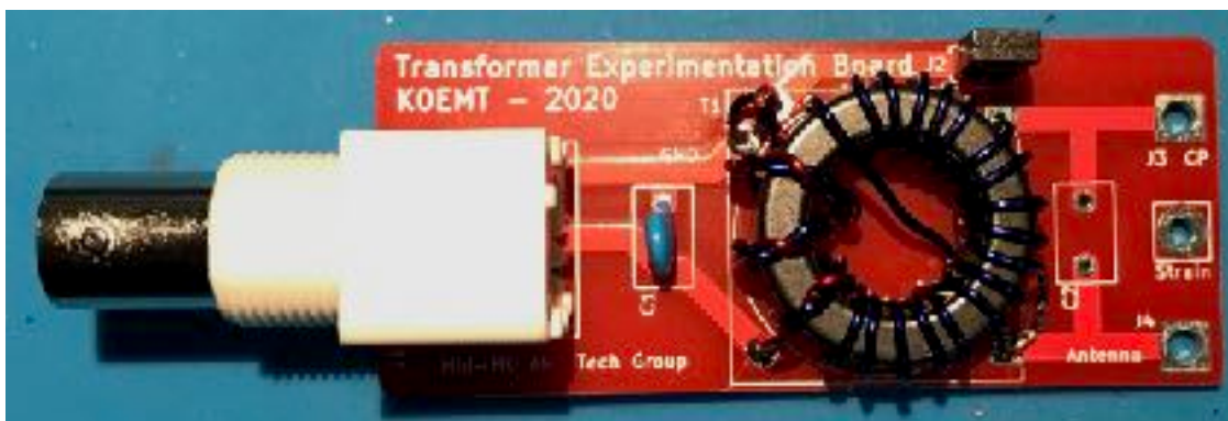
18-AWG enamel coated wire was used.
